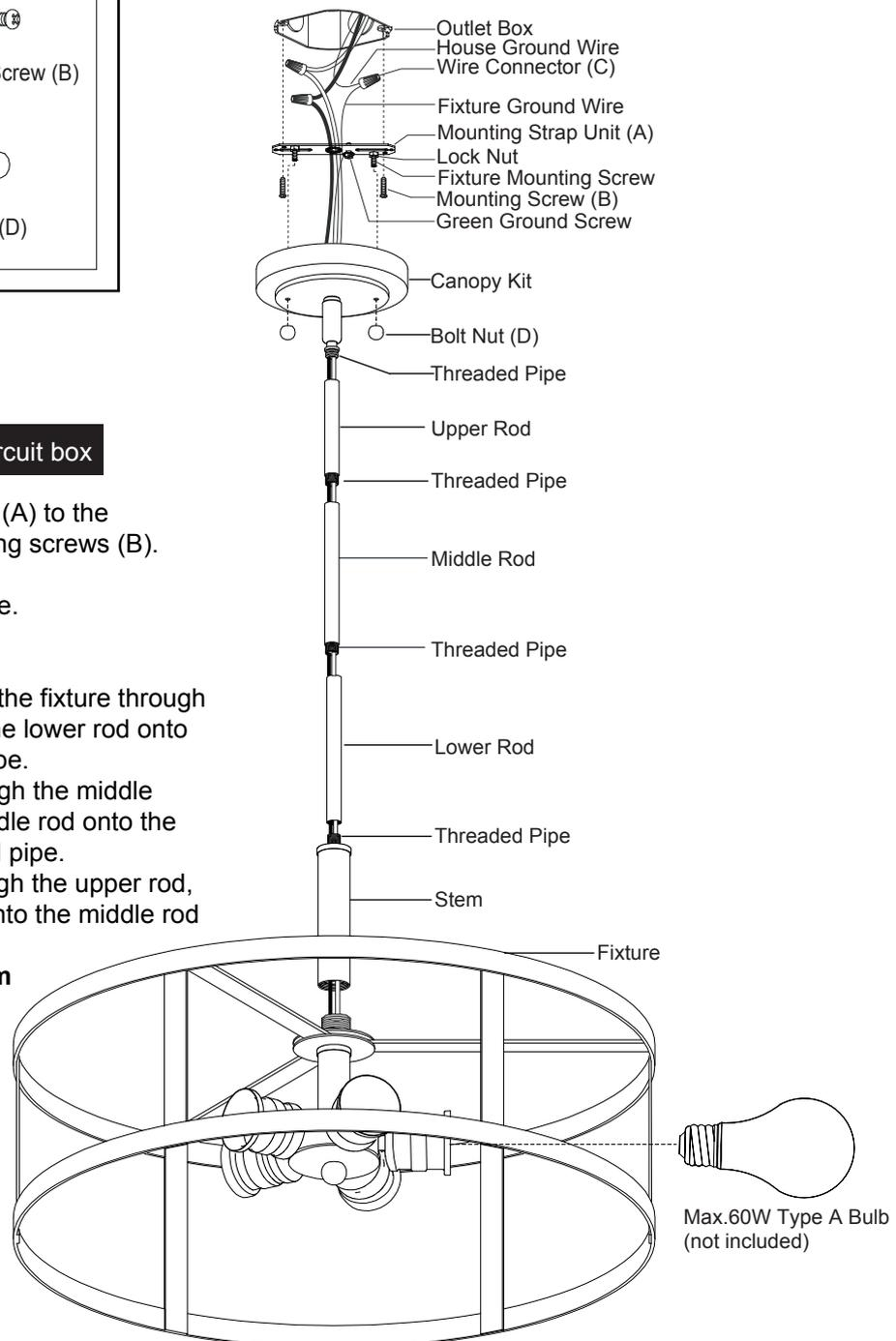
5. Pull out the source wires from the outlet box. Make wire connections using wire connectors (C) as follows:
